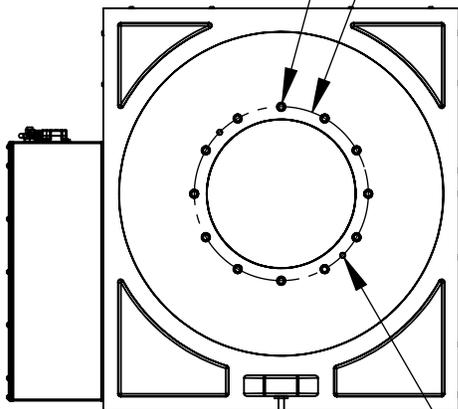
2X  $\varnothing .42in$  [10.7mm]  $\nabla 1.06in$  [26.9mm]
