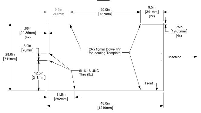
To accommodate the large variation in size and shape of material that can be loaded by the APL, use the following guidelines and table dimensions to make your own part specific templates
