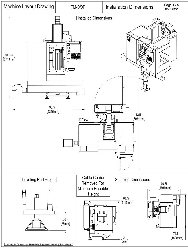
Maintain 3 feet [915mm] clearance to the nearest obstruction around all sides of machine perimeter for maintenance access
