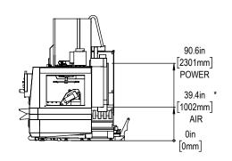
Maintain 3 feet [915mm] clearance to the nearest obstruction around all sides of machine perimeter for maintenance access
