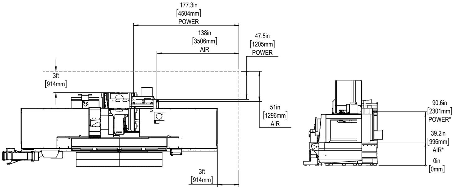
Maintain 3 feet [915mm] clearance to the nearest obstruction around all sides of machine perimeter for maintenance access
