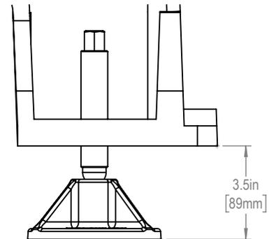
\*All Height Dimensions Based on Suggested Leveling Pad Height
