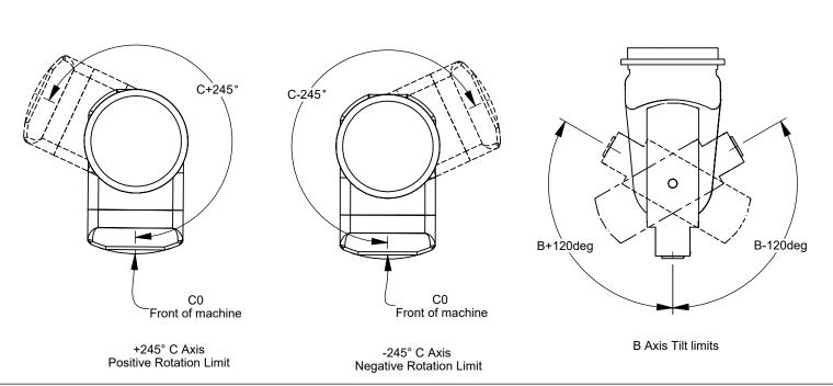
Isometric view of B & C Axis gimbal head for visual reference
