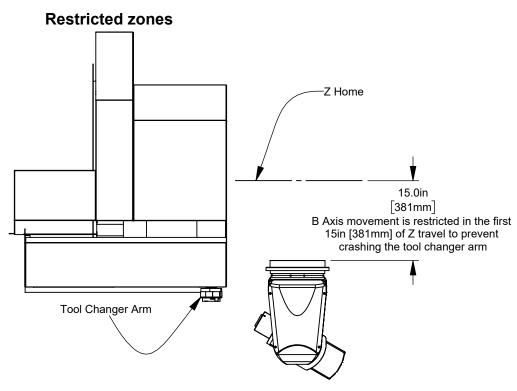
In addition to the tool changer interference zone, the machine has restricted zones between the gimbal head and fixed machine elements
