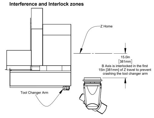
In addition to the tool changer interference zone, the machine has restricted zones between the gimbal head and fixed machine elements
