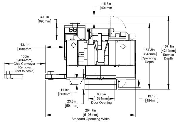
Maintain 3 feet [915mm] clearance to the nearest obstruction around all sides of machine perimiter for maintenance access
