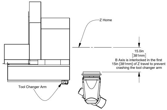
In addition to the tool changer interference zone, the machine has restricted zones between the gimbal head and fixed machine elements
