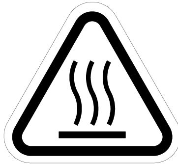
Fig. 4 (c) High-temperature warning label
