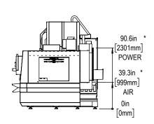
Maintain 3 feet [915mm] clearance to the nearest obstruction around all sides of machine perimeter for maintenance access
