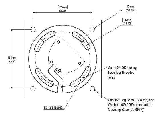
\*IF NOT USING MOUNTING BASE (09-0957), SELECT THE APPROPRIATE HARDWARE TAILORED TO YOUR SPECIFIC MOUNTING SURFACE
