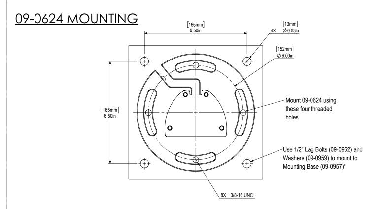
\*IF NOT USING MOUNTING BASE (09-0957), SELECT THE APPROPRIATE HARDWARE TAILORED TO YOUR SPECIFIC MOUNTING SURFACE
