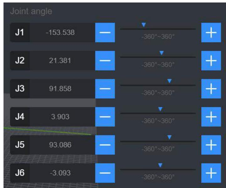
J1-J6 represent the axes from the first to the sixth of the robot. The text box displays the angle coordinate value of each corresponding axis position of the current robot in ° (angle).
