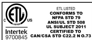
All Haas CNC machine tools carry the ETL Listed mark, certifying that they conform to the NFPA 79 Electrical Standard for Industrial Machinery and the Canadian equivalent, CAN/CSA C22.2 No. 73. The ETL Listed and cETL Listed marks are awarded to products that have successfully undergone testing by Intertek Testing Services (ITS), an alternative to Underwriters' Laboratories.
