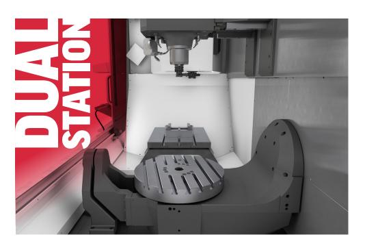
The UMC-1500-DU0 features a large 32" x 18" (813 mm x 457 mm) stationary T-slot table on the left that allows rigid setups for heavy material removal operations, using industrystandard table vises. The stationary table is also perfect for setting up first operations, or for machining the 6th side of your completed 5-axis parts.
