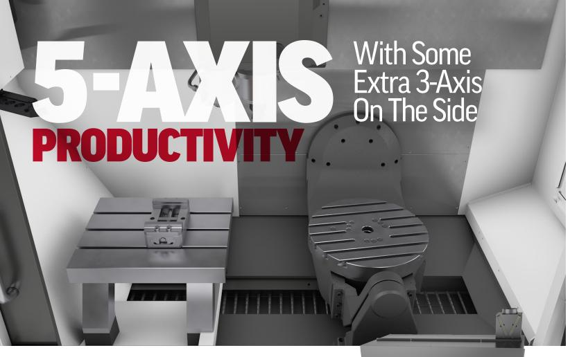
The Haas **UMC-1500-DUO** is like having two machines in one: a powerful 5-axis universal machining center, and a versatile 3-axis vertical machining center. We've taken our industry-leading UMC-750 universal machining center, expanded its X-axis travel, and added a stationary 32" x 18" (813 x 457 mm) T-slot table next to the dual-axis trunnion.
