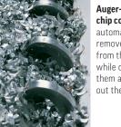
Auger-style chip conveyor automatically removes chips from the machine, while compressing them and wringing out the coolant.
