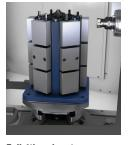
Full 4th-axis rotary provides high-accuracy positioning for tombstones and 3+1 work, as well as simultaneous 4th-axis motion for contouring and complex parts.
