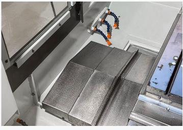
Steeply sloped way covers and angled internal sheet metal funnel chips into the side troughs, and powerful front washdown nozzles flush them to the rear of the machine. Rear chip discharge allows machines to be placed side-by-side to maximize shop space, and provides easy side access for automation systems.
