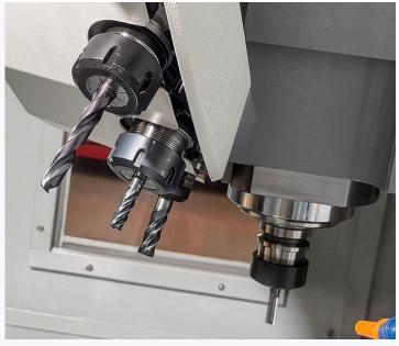
Each DC series machine is equipped with a **high-performance grease-packed spindle powered by a reliable Haas inline direct-drive system**. The spindle cartridge is liquid cooled for thermal stability. The Haas inline direct-drive system provides high accel/decel rates to minimize cut-to-cut times.
