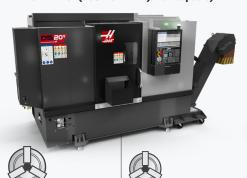
8.3" (210ER0 mm) Chuck 4000 rpm A2-6 Spindle Nose 2.5" (64 mm) Bar Capacity
