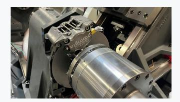
The mechanical disc brake on the C-Axis provides 140 ft-lb (190 Nm) of holding torque for off center milling and drilling.
