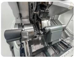
Each SB Series lathe is equipped with a robust 12-station BMT65 turret that accepts industry-standard base-mount tooling, as well as axial and radial driven live tools for secondary milling, drilling, and tapping operations.
