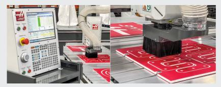
**SR SERIES SHEET ROUTERS** are equipped with the same powerful, easy-to-use Haas control found on every machine we build, and they come standard with a built-in vacuum dust collection system to remove chips, swarf, and dust produced during machining, keeping your shop cleaner, and reducing exposure to airborne dust.
