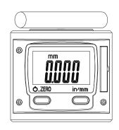
2. Place the bottom end on a ferrous surface to fix the height setter in place. Slowly descend the cutting tool onto the contact surface until the LED display lights up and reaches zero.
