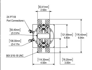
Total weight of the Single Pneumatic Gripper: About 7.5lbs [3.4kg]
