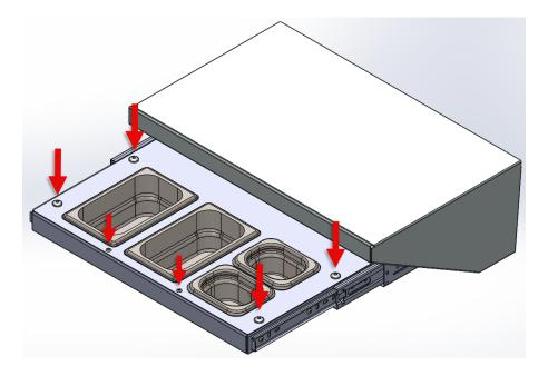
2. Replace existing tray with 09-0171 and tighten screws (6)
