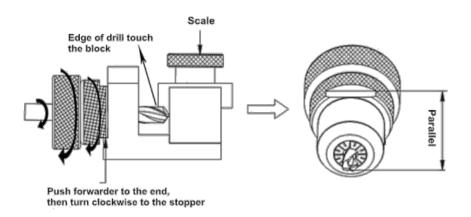
Attention: If the cutting lip is downward, must increase the scale of web adjustment shelf. If it is upward, please decrease the scale of the web adjustment shelf.
