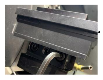
You now have access to the wedge clamp bolts. Clamp the tool block into the turret or holder.
