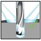
2) In case of external coolant, cutting depth must be 3XD or less.
