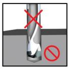
3) Dry cutting is not recommended. Limited applicability in cast iron materials, minimum quantity lubrication (MQL) strongly recommended.
