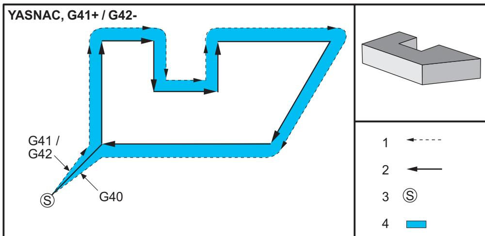
**F5.11:** Cutter Compensation, YASNAC Style, G42 with a Positive Tool Diameter or G41 with a Negative Tool Diameter: [1] Tool Path Actual Center, [2] Programmed Tool Path, [3] Start Point, [4] Cutter Compensation. G41 / G42 and G40 are commanded at the start and end of the tool path.
