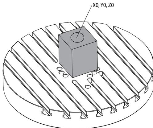
In the figure below, the actual workpiece is not located in this programmed position. The center of the workpiece is actually located at  $X_3, Y-2, Z_0$ , and is defined as G54.
