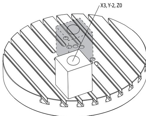
DWO is invoked in the figure below. The control knows the centers of rotation for the rotary table (MRZP), and the location of the workpiece (active work offset G54). The control uses this data to apply the appropriate offset adjustments to make sure that the proper toolpath is applied to the workpiece, as intended by the CAM-generated program. This eliminates the need to repost a program from the CAM system when the programmed and actual workpiece locations are different.
