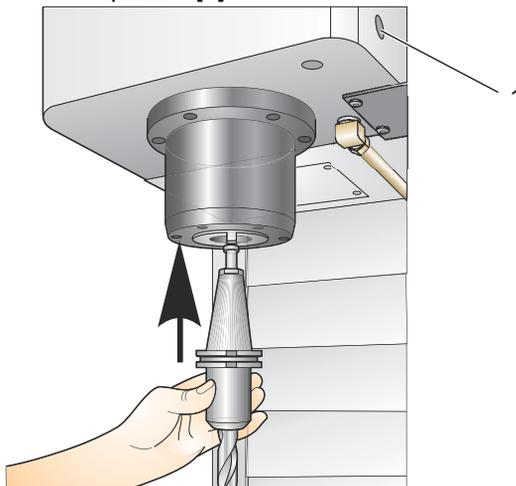
4. Turn the tool so that the two cutouts in the tool holder line up with the tabs of the spindle.
