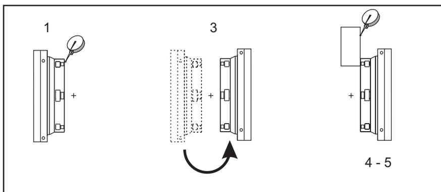
1. Jog the tilt axis until the rotary platter is vertical. Attach a dial indicator to the machine spindle (or other surface independent of table motion) and indicate the platter face. Set the dial indicator to zero.
