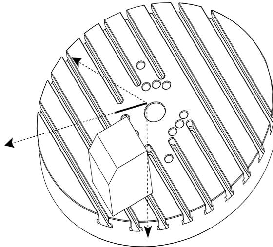
TCPC is invoked in Figure **F7.49**. The Haas CNC control knows the centers of rotation for the rotary table (MRZP), and the location of the workpiece (active work offset G54). This data is used to produce the desired machine motion from the original CAM-generated program. The machine follows an interpolated X-Y-Z path to create this edge, even though the program simply commands a single-axis move along the Y Axis.
