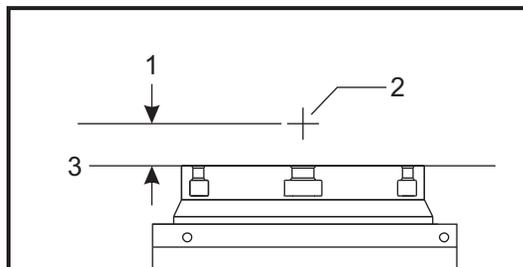
**F6.19:** Tilt Axis Center-of-Rotation Illustrated Procedure. Numeric labels in this diagram correspond to the step numbers in the procedure.
