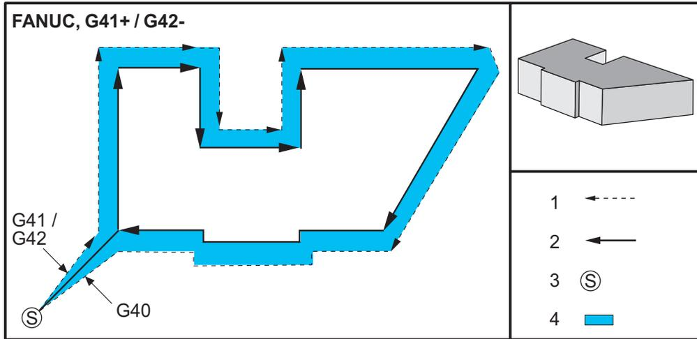
**F5.13:** Cutter Compensation, FANUC Style, G42 with a Positive Tool Diameter or G41 with a Negative Tool Diameter: [1] Tool Path Actual Center, [2] Programmed Tool Path, [3] Start Point, [4] Cutter Compensation. G41 / G42 and G40 are commanded at the start and end of the tool path.
