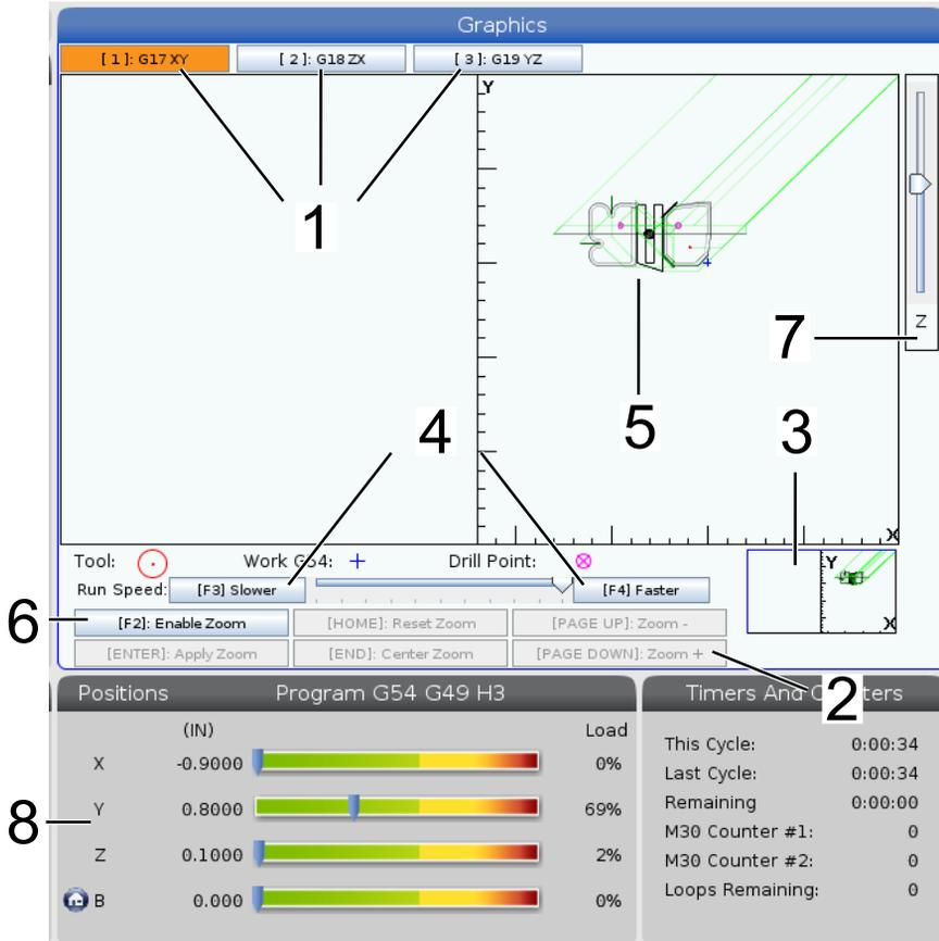
1. **Axis Planes** Press **[1]** to view the graphics in G17 plane, press **[2]** for G18 plane or press **[3]** to view in G19 plane.
