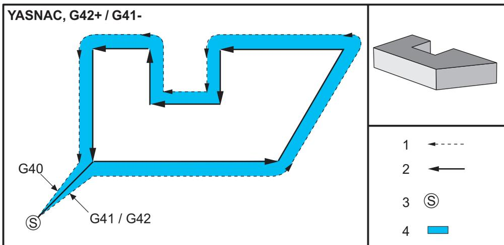
**F5.12:** Cutter Compensation, FANUC Style, G41 with a Positive Tool Diameter or G42 with a Negative Tool Diameter: [1] Tool Path Actual Center, [2] Programmed Tool Path, [3] Start Point, [4] Cutter Compensation. G41 / G42 and G40 are commanded at the start and end of the tool path.
