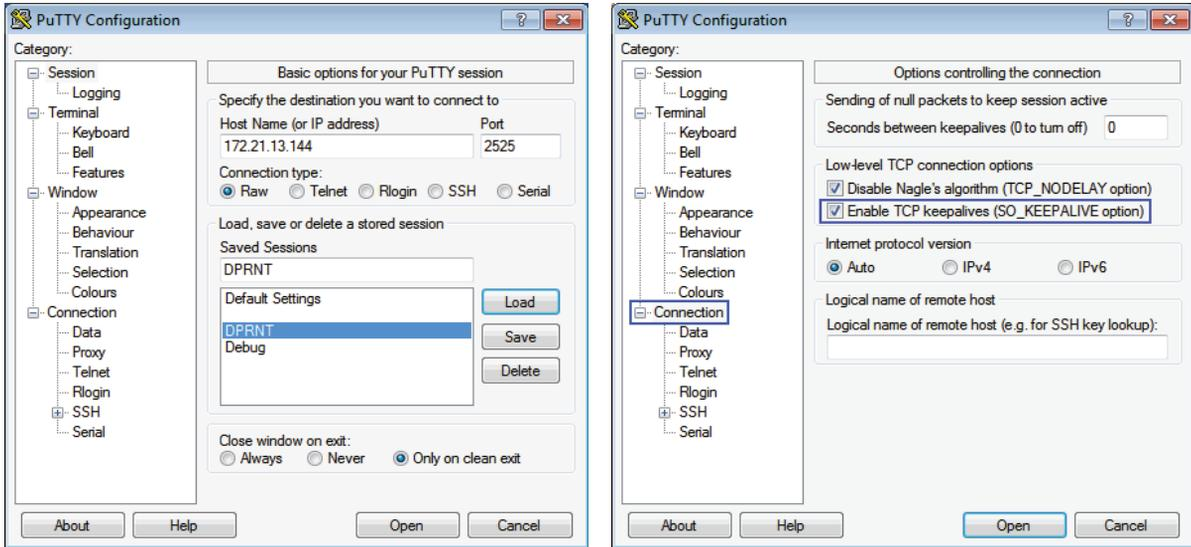
To check the connection, type `?Q100` in the PuTTY terminal window. If the connection is active, the machine control responds with `SERIAL NUMBER, XXXXXX`, where `XXXXXX` is the machine's actual serial number.
