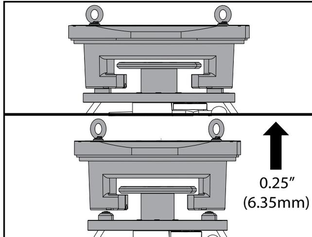
3. Lift the pallet approximately 0.25" (6.35mm) to position it above the load station pins, but below the load station lock plate. Pull the pallet towards you until it has cleared the load station.
