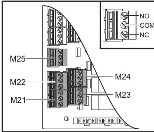
**F8.3:** M-Fin Circuit at P8 on the Main I/O PCB. Pin 3 is the M-Fin input and interacts with input number 18 in the control. Pin 1 is the M-Fin output and interacts with output number 4 on the control.
