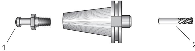
2. Clean the tool holder taper body (the part that goes into the spindle) with a lightly oiled rag to leave a film, which helps prevent rusting.
