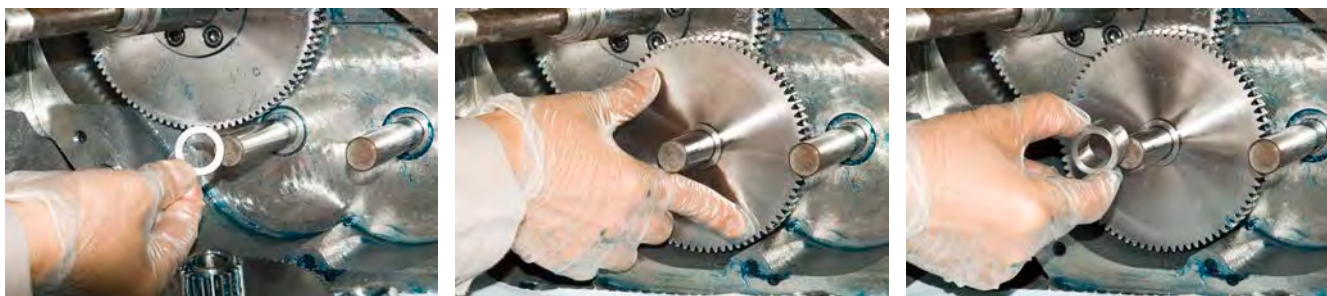
Install spacers and gear on second shaft
