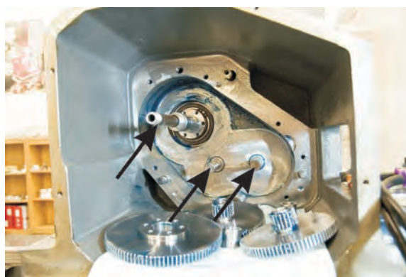
Lubricate the three gearbox shafts
