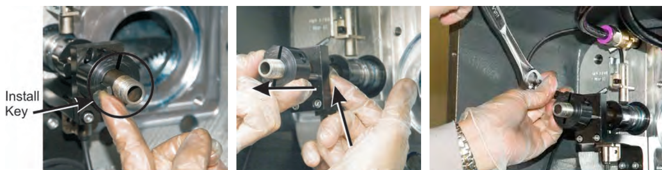
Install the key and set collar position
