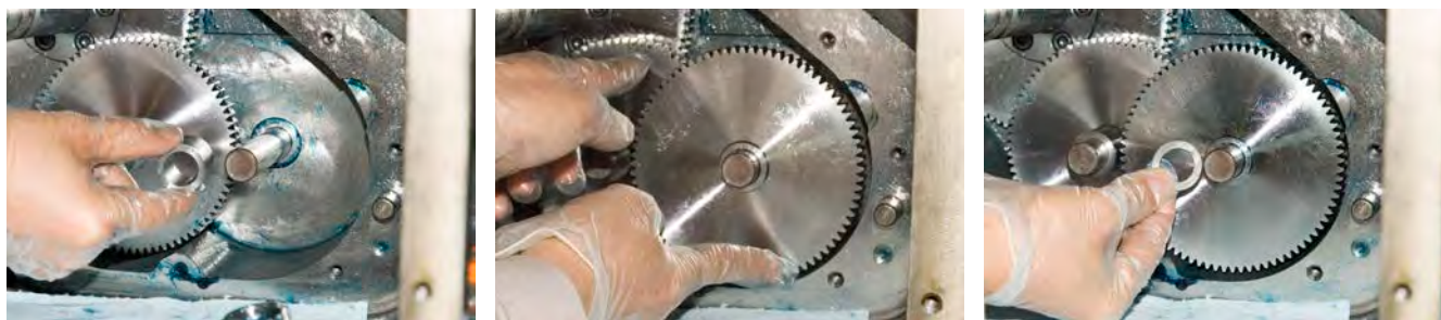
Install spacers and gear on the third shaft.
