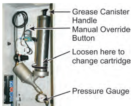
Grease System Assembly
