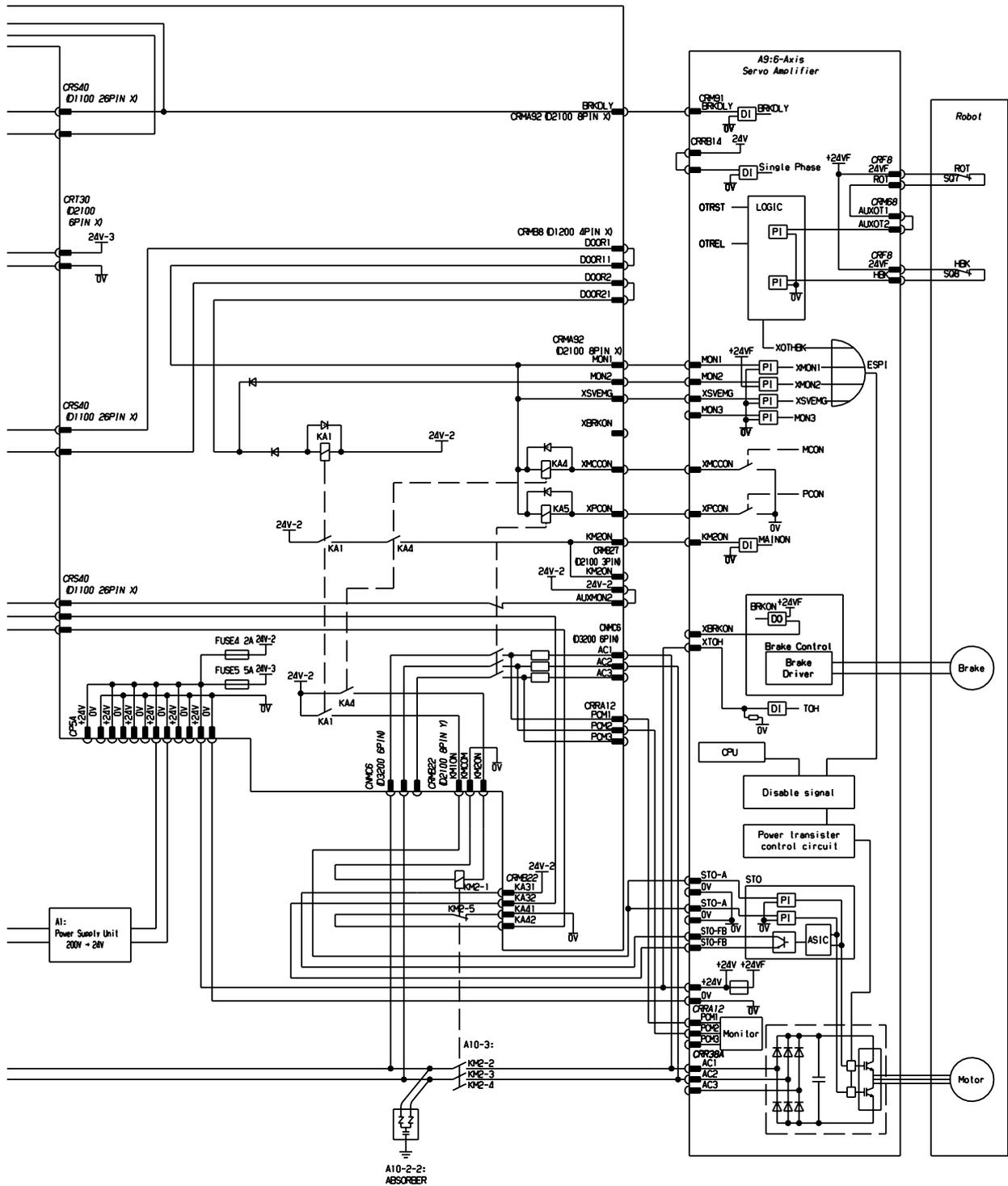
R-30iB Mate E-STOP Board Connector Table
