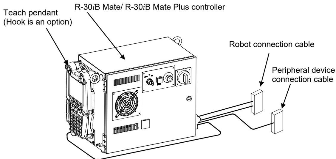
Fig.5.2.2 Assemble at installation
