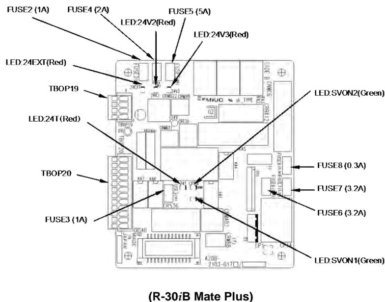
Fig.3.6 (c) Fuse on the emergency stop board
