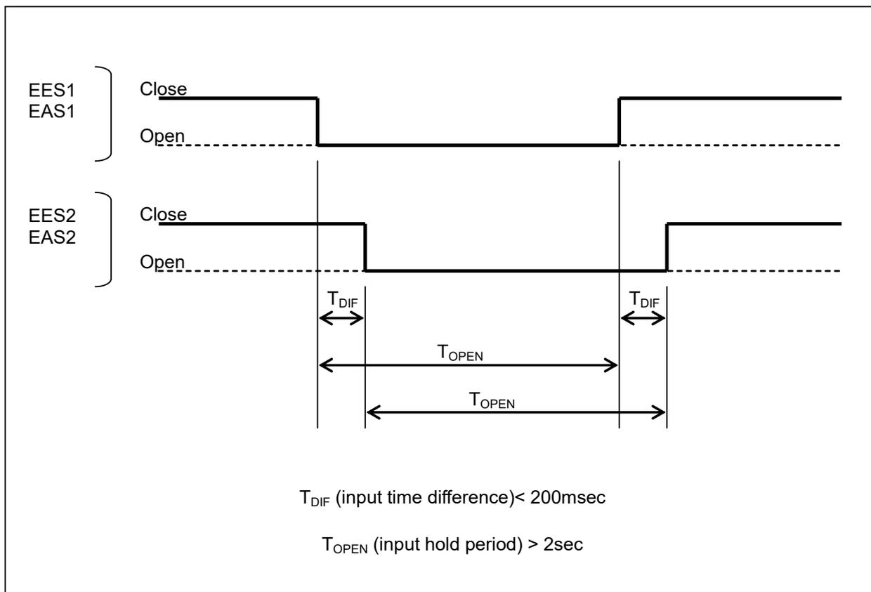
**Fig.3.3.4(c) Input timing of duplicate safety signals**
