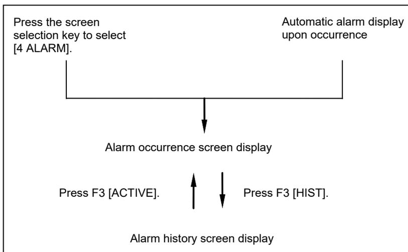
Fig.3.2 Alarm occurrence screen and alarm history screen display procedure
