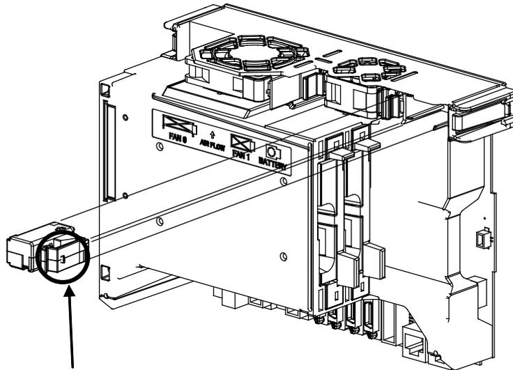
Insert the unit until the latch snaps into the case
