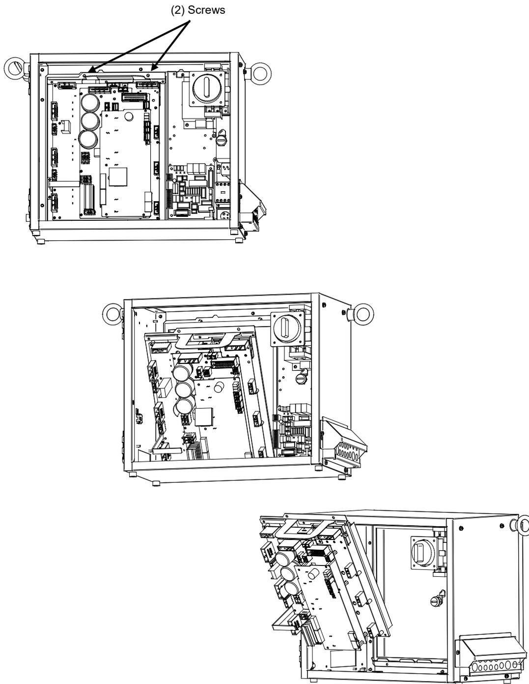
Fig.8.7 Replacing the servo amplifier
