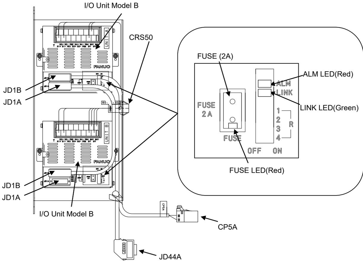
Fig.6 Sensor I/F unit for CR-4iA, CR-7iA
