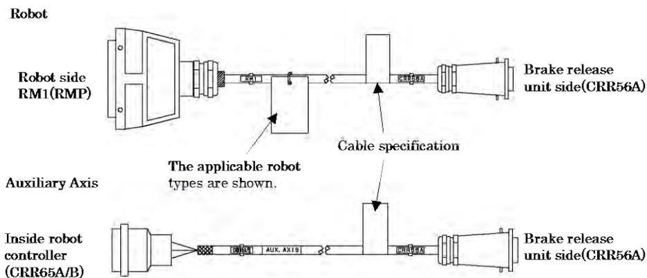
**Fig.E.2 Brake release unit connection cable**
