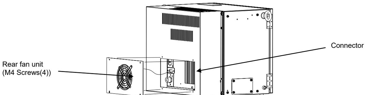
Fig.8.10.1(b) Replacing the rear fan unit
