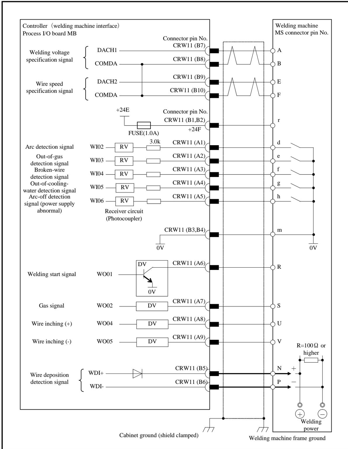
**Pin-to-pin connection between CRW11 connector and welding machine connector (FANUC interface)
