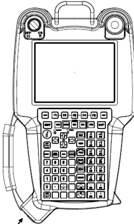
Detach or attach the cable by rotating the connector retaining ring.
