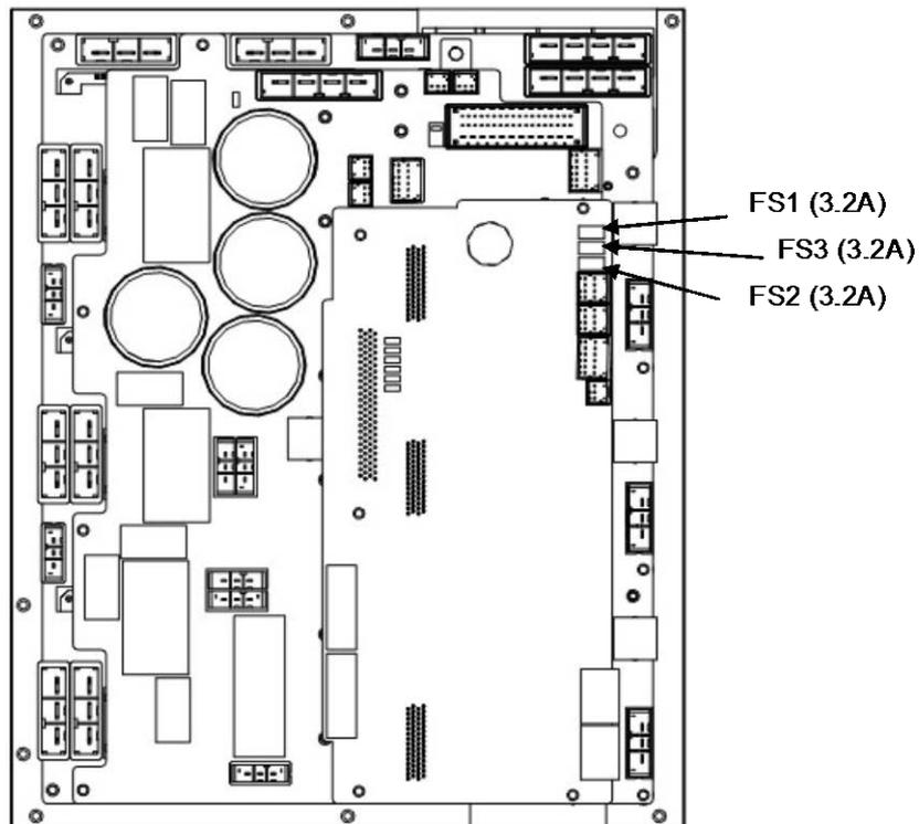
Fig.3.6(b) Fuse on the servo amplifier
