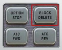
% O00001 (MILL FORMAT); N1 (NOTES) G00 G17 G20 G40 G49 G54 G64 G80 G90 G94 G98 G100; G53 Z0.; T1 M06; X0. Y0. S1000 M03; G43 H01 Z1. M08; (BEGIN TOOL BODY); /G83 X3. Y2. Z-1. R.1 Q.25 F3. (END TOOL BODY); G00 G80 Z1. M09; G49 G53 Z0.; M01
