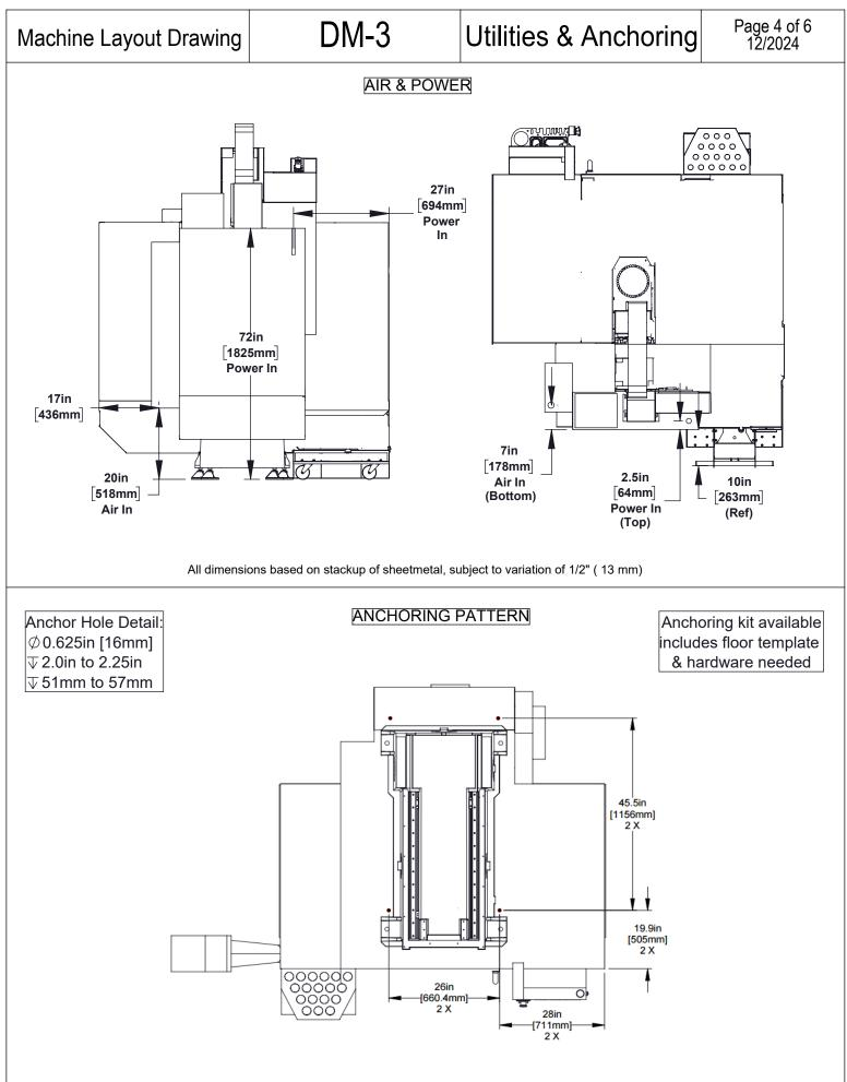
Note: Machine must be placed on one continous concrete slab. Slab should extend 12in [305mm] beyond anchor holes in all directions
