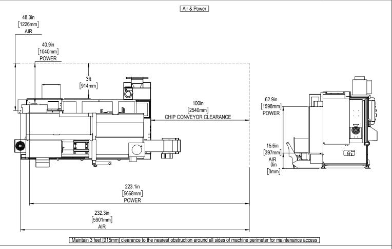
Note: Machine must be placed on one continous concrete slab. Slab shiould extend 12in [305mm] beyond anchor holes in all directions
