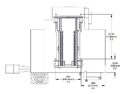
Note: Machine must be placed on one continous concrete slab. Slab should extend 12in [305mm] beyond anchor holes in all directions
