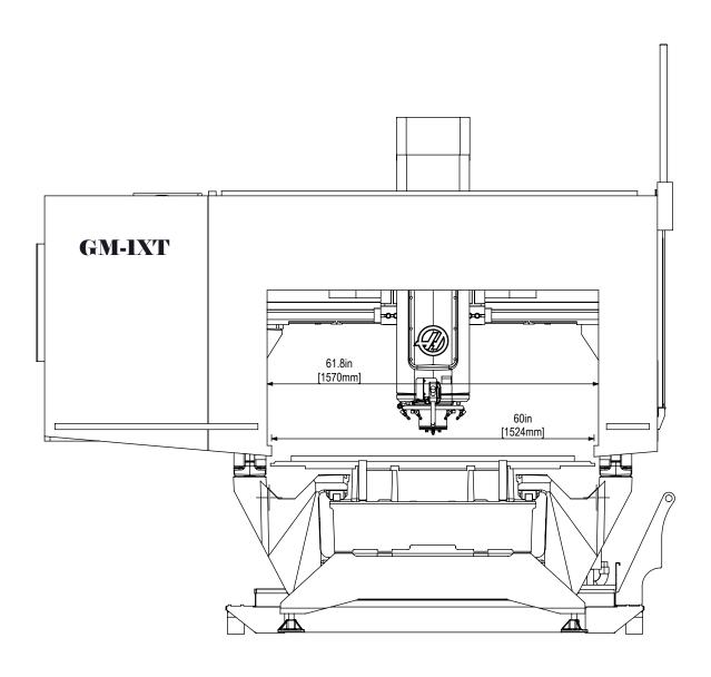
IF THE PART IS RAISED 2.5 INCHES (63.5MM) FROM THE TABLE TOP, A PART MEASURING 61.8 INCHES (1570mm) WIDE, MAY BE CLEARED THRU THE COLUMNS.
