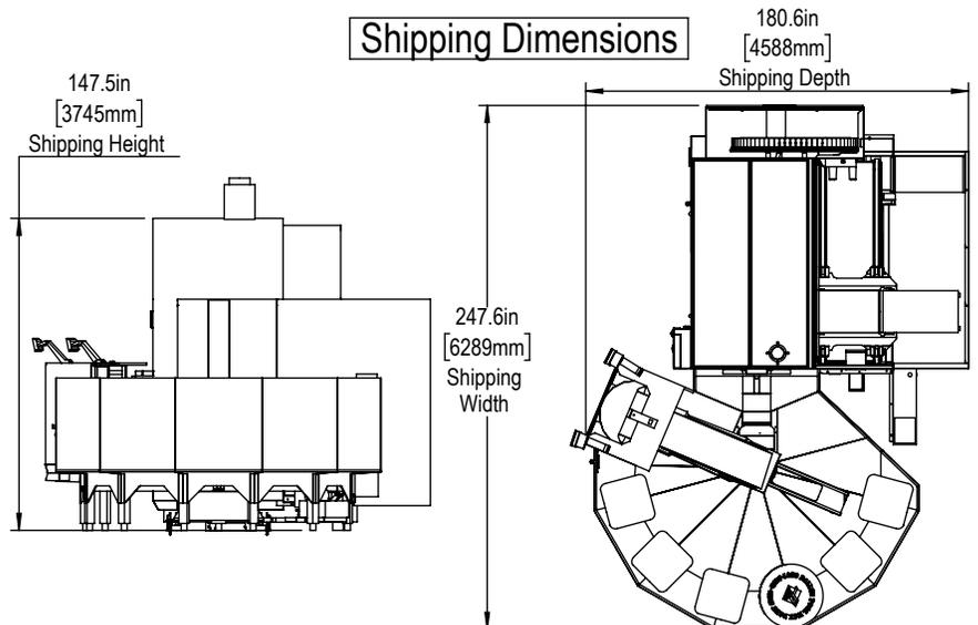
\*All Height Dimensions Based on Suggested Leveling Pad Height
