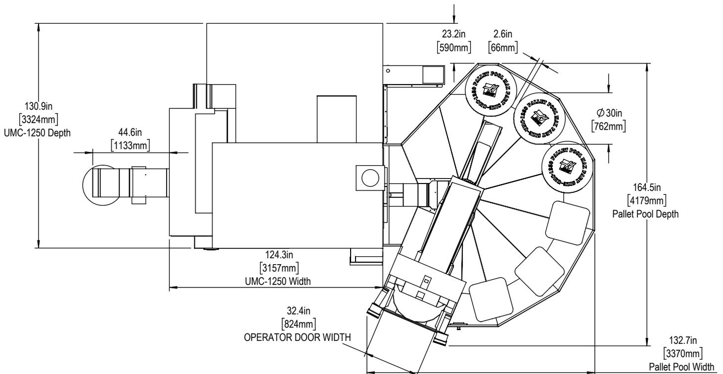
Maintain 3 feet [915mm] clearance to the nearest obstruction around all sides of machine perimeter for maintenance access
