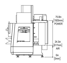
Maintain 3 feet [915mm] clearance to the nearest obstruction around all sides of machine perimeter for maintenance access
