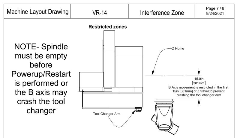
In addition to the tool changer interference zone, the machine has restricted zones between the gimbal head and fixed machine elements
