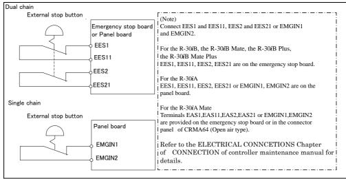
Fig. 3.1 Connection diagram for external emergency stop button
