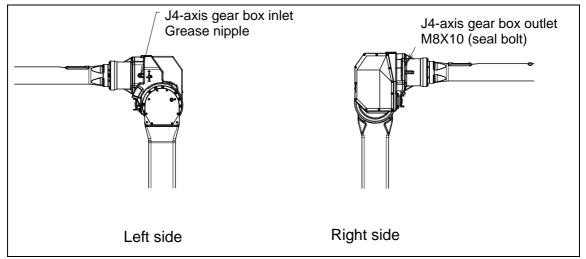
Fig. 7.3.3.2 Replacing grease of the J4-axis gearbox (When the Seal Bolt is M8x10)
