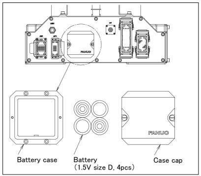
Fig. 7.3.1 (a) Replacing the battery
