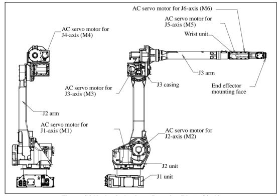
Fig. 3.1 (b) Mechanical unit configuration (M-710iC/12L)
