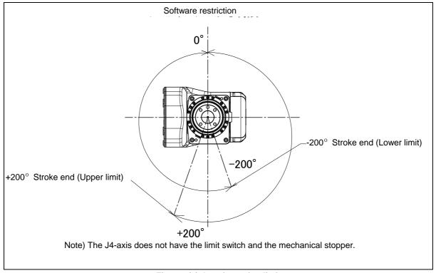
Fig. 3.3 (e) J4-axis motion limit
