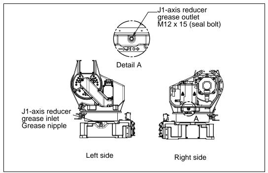
Fig. 8.3.2.1 (a) Replacing grease of the J1-axis reducer
