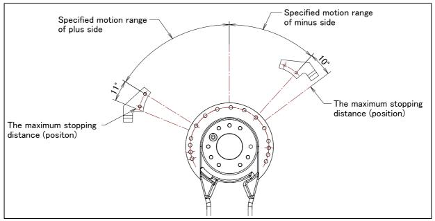
Fig. 6.2 (h) The maximum stopping distance of movable mechanical stopper
