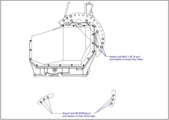
Fig. 6.2 (b) J2-Axis movable mechanical stopper
