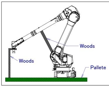
Fig. 1.1.1 Example of securing the arm during transportation when an end effector is attached
