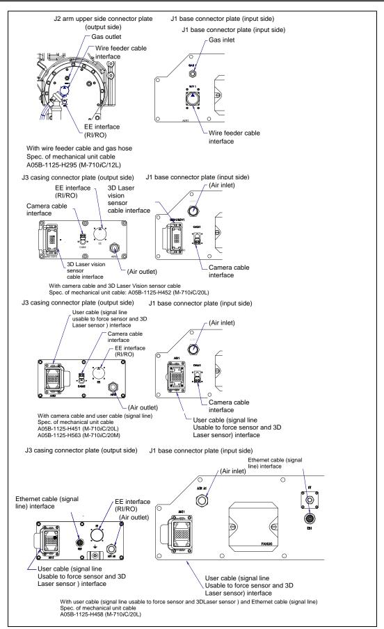
Fig. 5.3 (c) Interface for option cable 2/2
