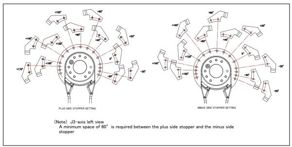
Fig. 6.2 (e) Attachment of J3-Axis movable mechanical stopper
