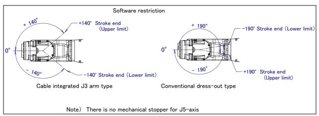
Fig. 3.3 (g) J5-axis motion limit (M-710iC/12L)
