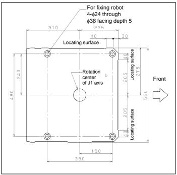
Fig. 1.2 Dimensions of the robot base
