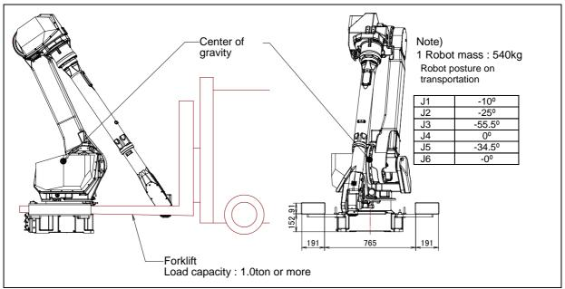
Fig. 1.1 (e) Transportation using a forklift (M-710iC/20L)
