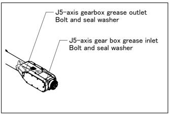
Fig. 7.3.3.3 Grease replacement procedure for the J5-axis gearbox
