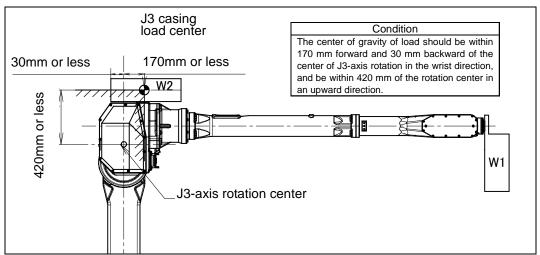
Fig. 3.5 (a) J3 casing load condition (M-710iC/20L/20M)
