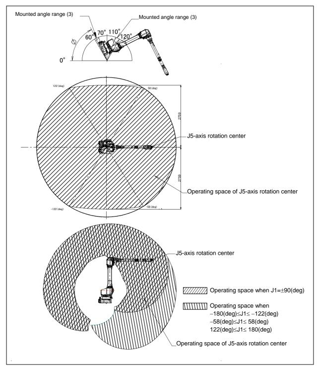
Fig. 3.7 (c) Operating space for mounted angle range (3)  $(60^{\circ}<\phi\leq70^{\circ},\,110^{\circ}\leq\phi<120^{\circ})$  (M-710iC/20L)
