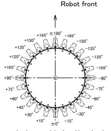
(Note) This figure is drawn with the J1-axis viewed from above. The dog of the J1-axis is placed in the same position as with the mechanical stopper.
