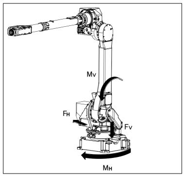
Fig. 1.2.1 (b) Force and moment during Power-Off Stop
