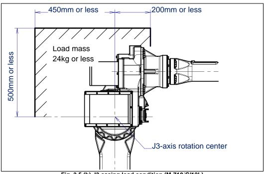
Fig. 3.5 (b) J3 casing load condition (M-710iC/12L)
