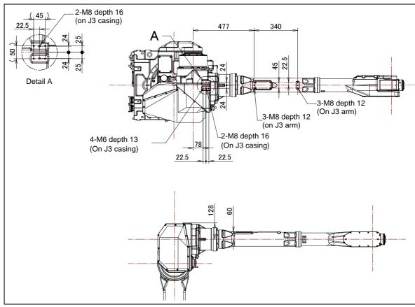
Fig. 4.2 (c) Equipment mounting surfaces (M-710iC/20M)
