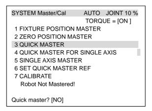
Select [4 QUICK MASTER FOR SINGLE AXIS]. The quick master for single axis screen will be displayed.
