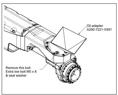
Fig. 8.3.2.3 (e) Oil adapter (supplying oil J5/J6-axis gearbox)
