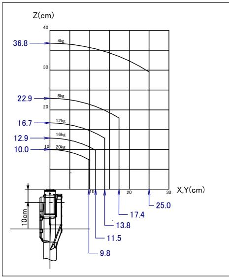
Fig. 3.4 (a) Wrist load diagram (M-710iC/20L/20M)
