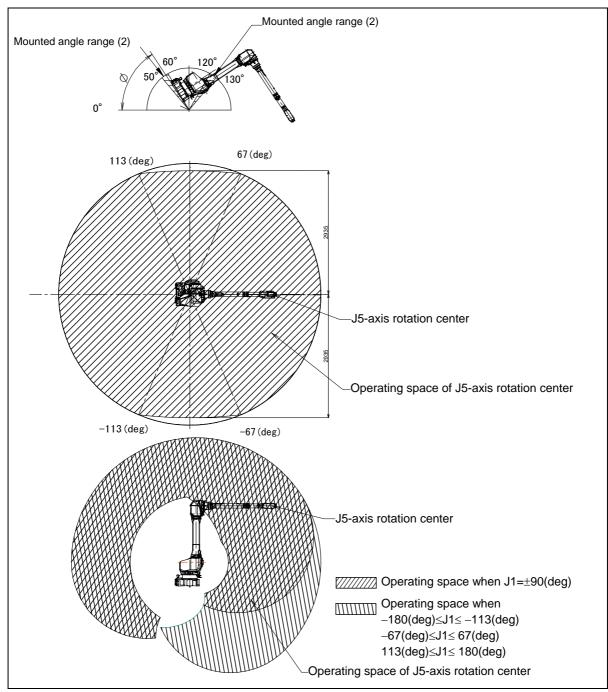
Fig. 3.7 (b) Operating space for mounted angle range (2)  $(50^{\circ} < \phi \le 60^{\circ}, 120^{\circ} \le \phi < 130^{\circ})$  (M-710*i*C/20L)
