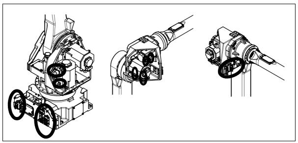
Fig. 7.2.3 (b) Connector Inspection points
