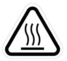
Fig. 10 (c) High-temperature warning label
