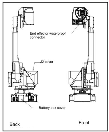
Fig. 11.2 Configuration of the Severe dust/liquid protection package of M-710iC/20L
