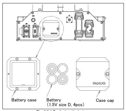
Fig. 8.3.1 Replacing the battery
