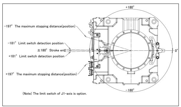
Fig. 3.3 (b) J1-axis motion limit
