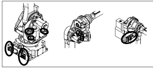
Fig. 8.2.5 (b) Connector Inspection points
