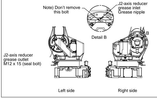
Fig. 8.3.2.1 (b) Replacing grease of the J2-axis reducer
