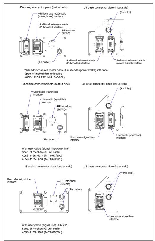
Fig. 5.3 (b) Interface for option cable 1/2
