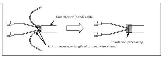
Fig. 5 Treatment method of end effector (hand) cable
