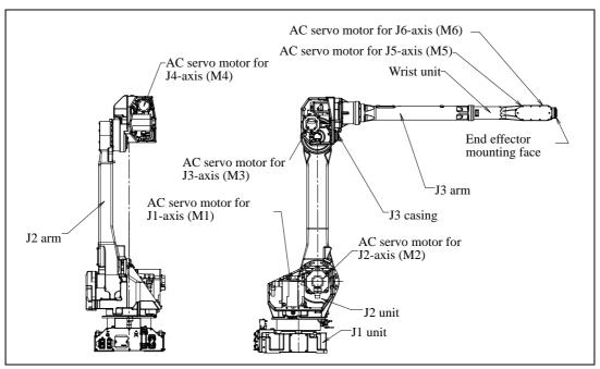
Fig. 3.1 (a) Mechanical unit configuration (M-710iC/20L/20M)
