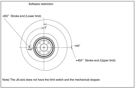
Fig. 3.3 (h) J6-axis motion limit (M-710*i*C/20L/20M)
