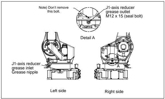
Fig. 7.3.3.1 (a) Replacing grease of the J1-axis reducer
