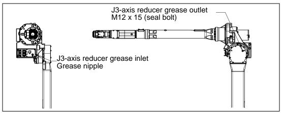
Fig. 8.3.2.1 (c) Replacing grease of the J3-axis reducer
