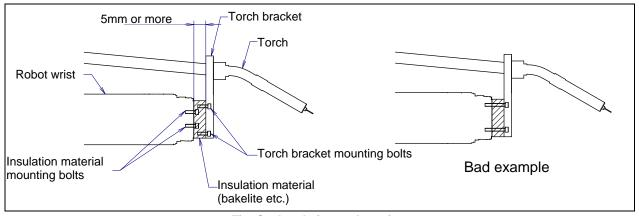
Fig. C.1 Insulation at the wrist
