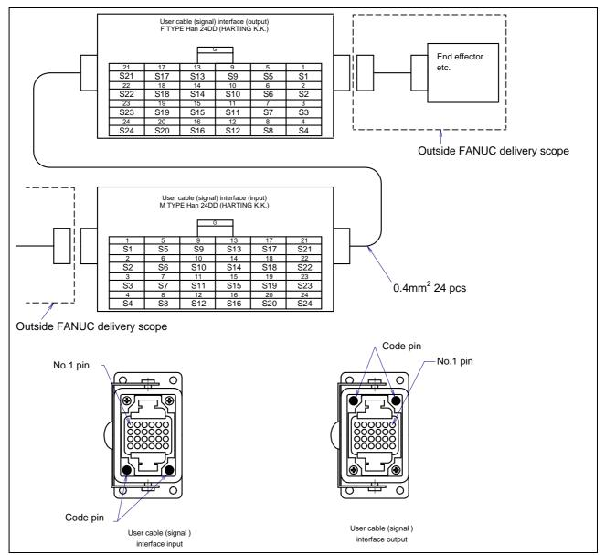
Fig. 5.3 (g) Pin layout for user cable (signal line) (AS) interface and code pin layout (option)
