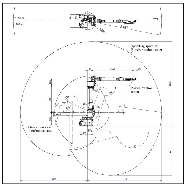
Fig. 3.2 (b) Operating space (M-710iC/12L)
