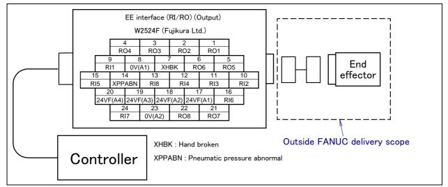
Fig. 5.3 (e) Pin layout for EE interface (RI/RO) (option)
