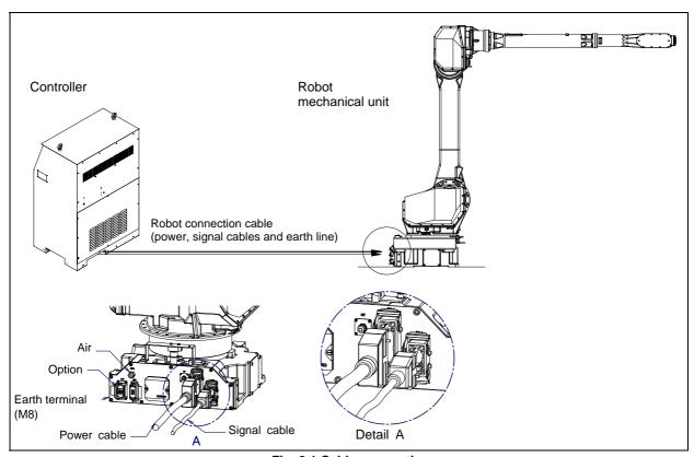
Fig. 2.1 Cable connection
