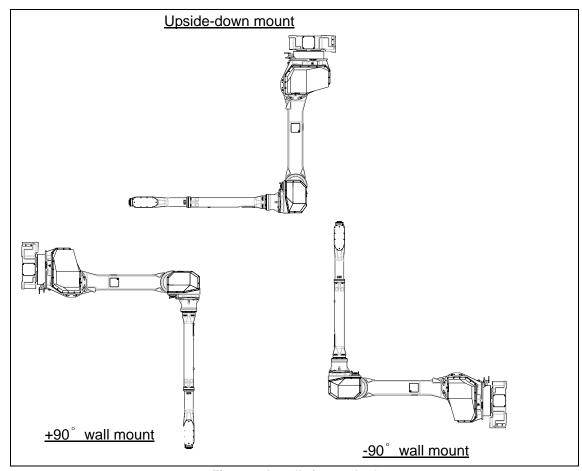
Fig. 7.3.3 Installation method
