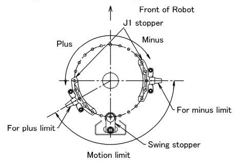
Fig. 6.2 (a) Mechanical stopper and motion limit of J1-axis (Option)
