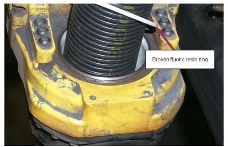
Fig. 8.2.4 (b) Failure of the fluoric resin ring
