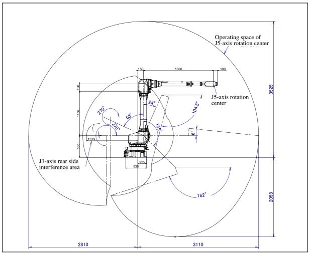
Fig. 3.2 (a) Operating space (M-710iC/20L)
