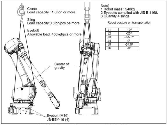
Fig. 1.1 (b) Transportation using a crane (M-710*i*C/20L)
