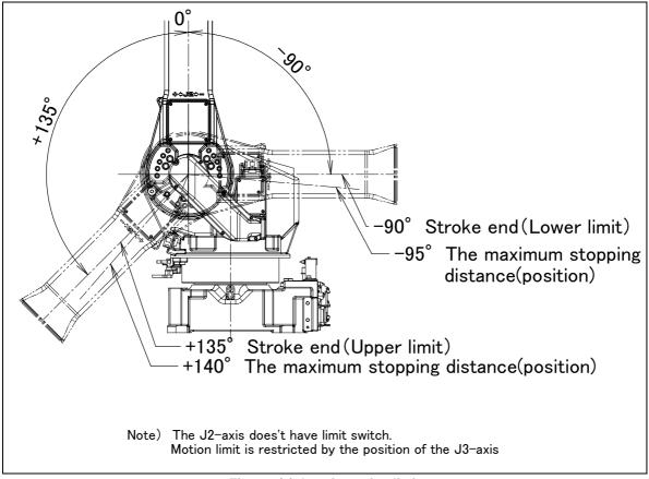
Fig. 3.3 (c) J2-axis motion limit
