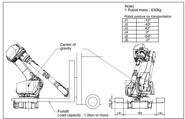
Fig. 1.1 (g) Transportation using a forklift (M-710iC/20M)
