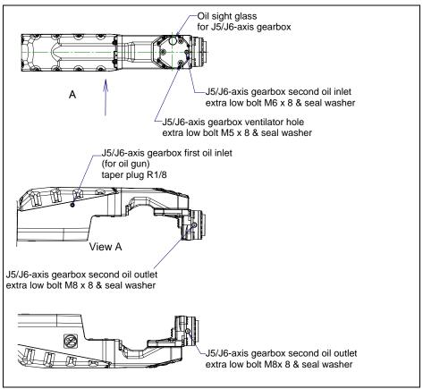
Fig. 8.3.2.3 (b) Oil inlet and outlet
