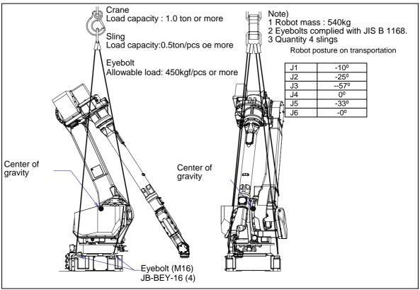
Fig. 1.1 (c) Transportation using a crane (M-710iC/12L)
