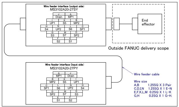
Fig. 5.3 (I) Pin layout for LINCOLN wire feeder power supply (W/F) interface (option)
