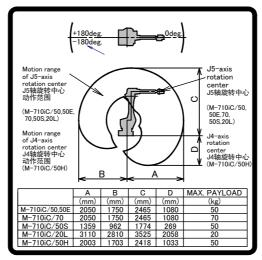
Fig. 10 (f) Operating space and payload label (Example of M-710iC/20L)
