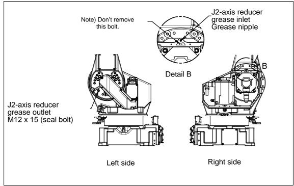
Fig. 7.3.3.1 (b) Replacing grease of the J2-axis reducer
