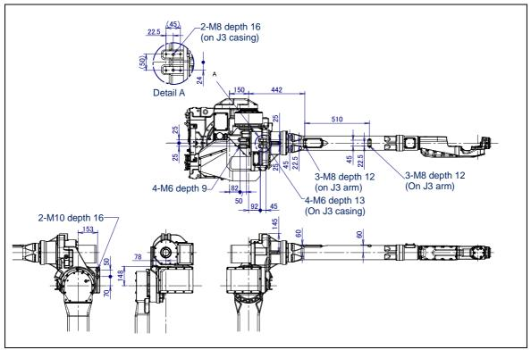
Fig. 4.2 (b) Equipment mounting surfaces (M-710iC/12L)
