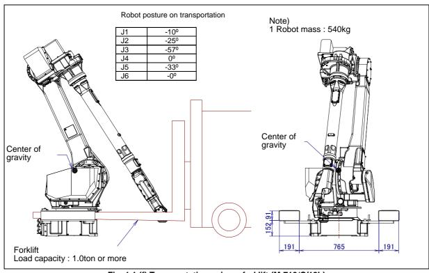
Fig. 1.1 (f) Transportation using a forklift (M-710iC/12L)
