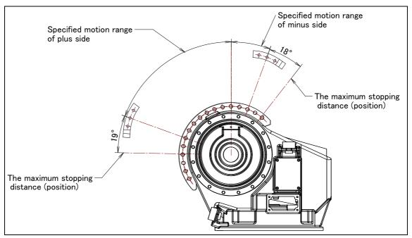
Fig. 6.2 (g) The maximum stopping distance of movable mechanical stopper (J2-axis)
