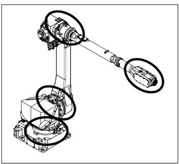
Fig. 7.2.1 Check parts of oil seepage
