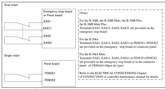
Fig. 3 (b) Connection diagram for the signal of safety fence
