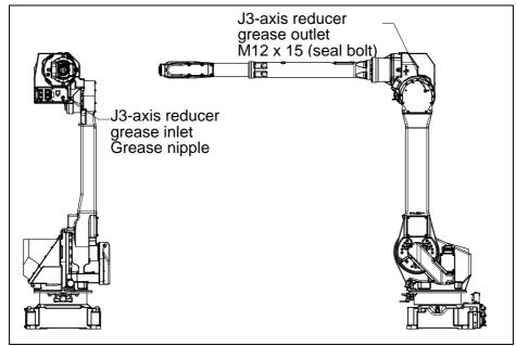
Fig. 7.3.3.1 (c) Replacing grease of the J3-axis reducer
