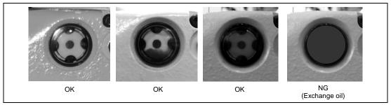
Fig. 8.2.3 The extent of oil deterioration
