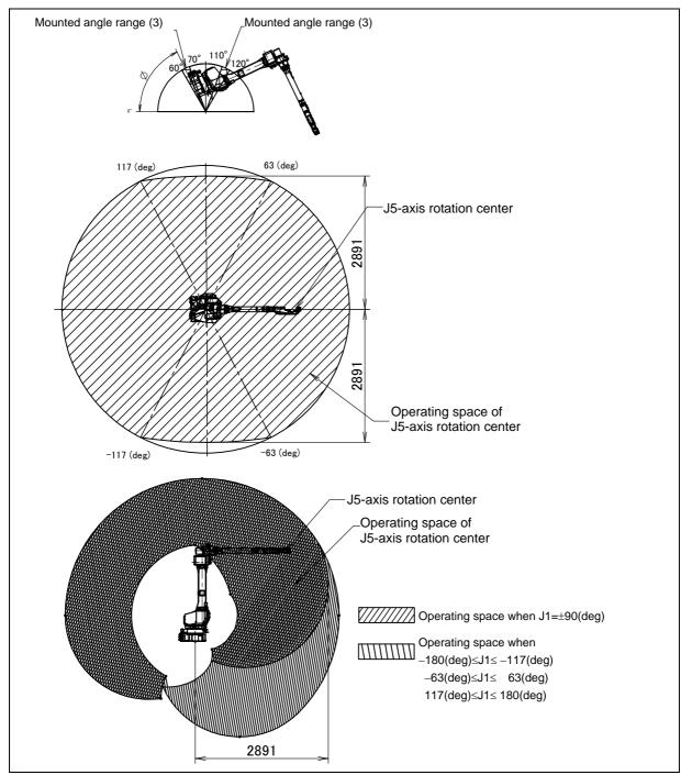
Fig. 3.7 (g) Operating space for mounted angle range (3)  $(60^{\circ} < \phi \le 70^{\circ}, 110^{\circ} \le \phi < 120^{\circ})$  (M-710*i*C/12L)
