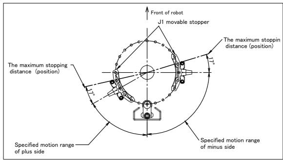
Fig. 6.2 (f) The maximum stopping distance of movable mechanical stopper (J1-axis)
