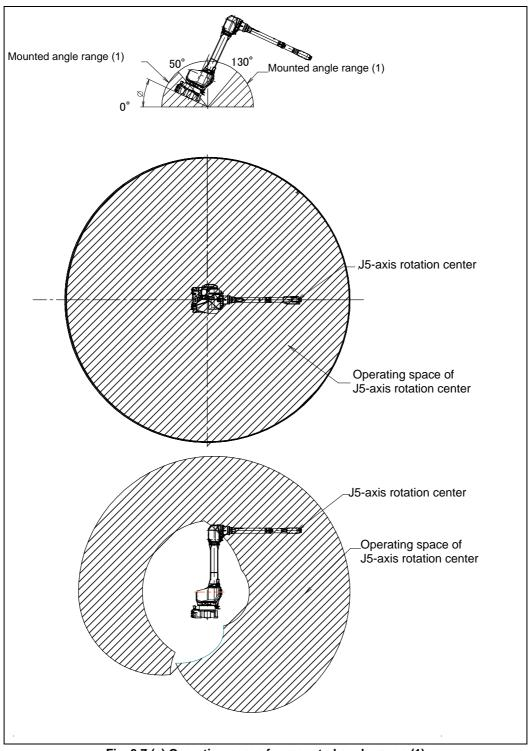
Fig. 3.7 (a) Operating space for mounted angle range (1)  $(0^{\circ} \le \phi \le 50^{\circ}, 130^{\circ} \le \phi \le 180^{\circ})$  (M-710*i*C/20L)
