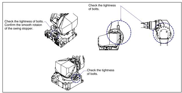
Fig. 8.2.6 Check of fixed mechanical stopper and adjustable mechanical stopper
