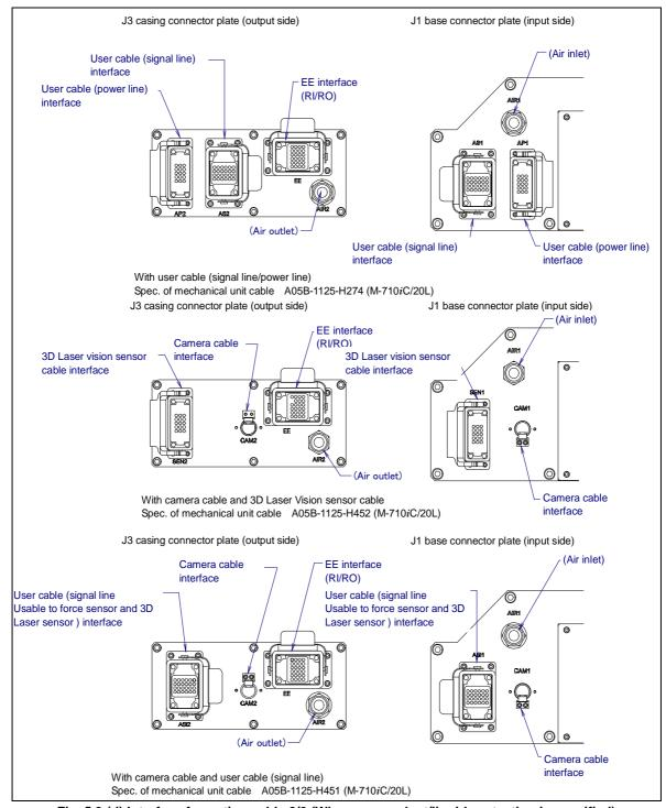
Fig. 5.3 (d) Interface for option cable 2/2 (When severe dust/liquid protection is specified)
