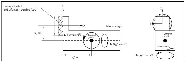
Fig. 4.3 Standard tool coordinate
