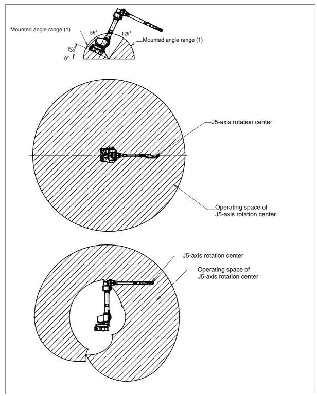
Fig. 3.7 (e) Operating space for mounted angle range (1)  $(0^{\circ} \le \phi \le 55^{\circ}, 125^{\circ} \le \phi \le 180^{\circ})$  (M-710*i*C/12L)
