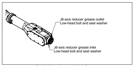
Fig.7.3.2 Greasing the J6-Axis Reducer
