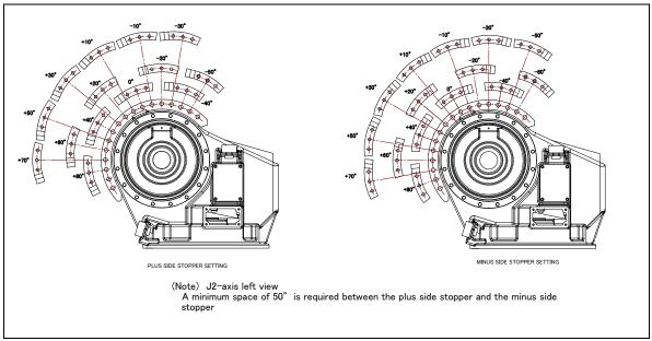
Fig. 6.2 (c) Attachment of J2-Axis movable mechanical stopper
