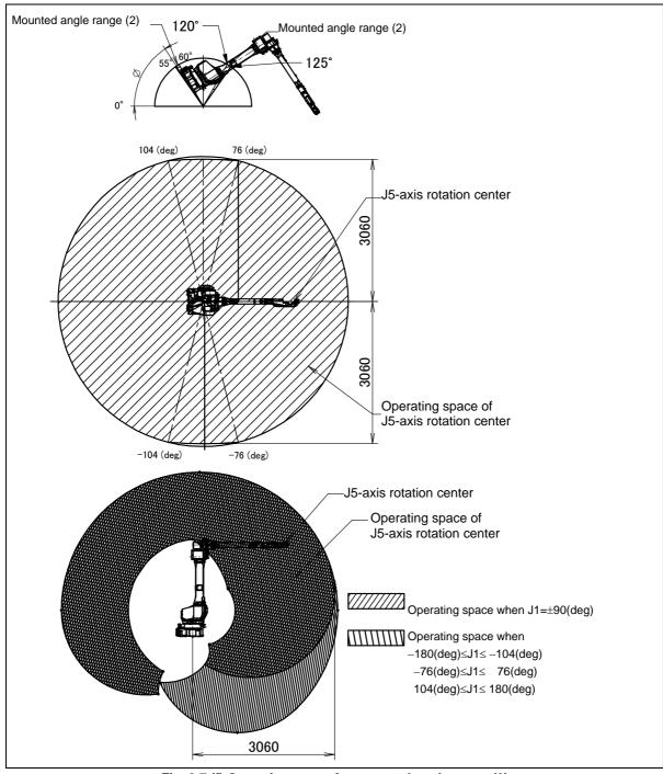
Fig. 3.7 (f) Operating space for mounted angle range (2)  $(55^{\circ} \le \phi \le 60^{\circ}, 120^{\circ} \le \phi \le 125^{\circ})$  (M-710*i*C/12L)
