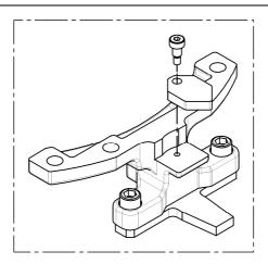
The dog of the J1-axis is attached to the mechanical stopper. At this time, use the screw hole of the mechanical stopper.
