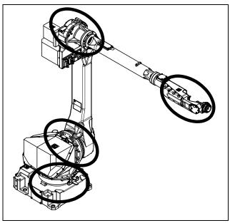
Fig. 8.2.1 Check parts of oil seepage
