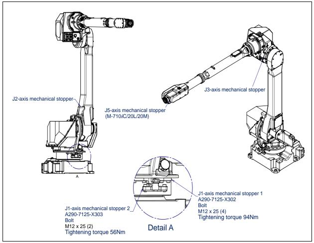
Fig. 3.3 (a) Position of mechanical stopper
