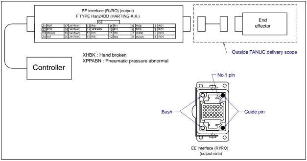
Fig. 5.3 (f) Pin layout for EE interface (RI/RO) (Severe dust/liquid protection package)
