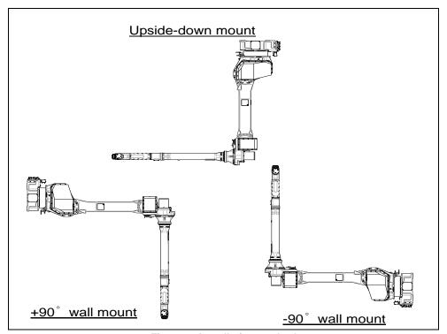
Fig. 8.3.2 Installation method
