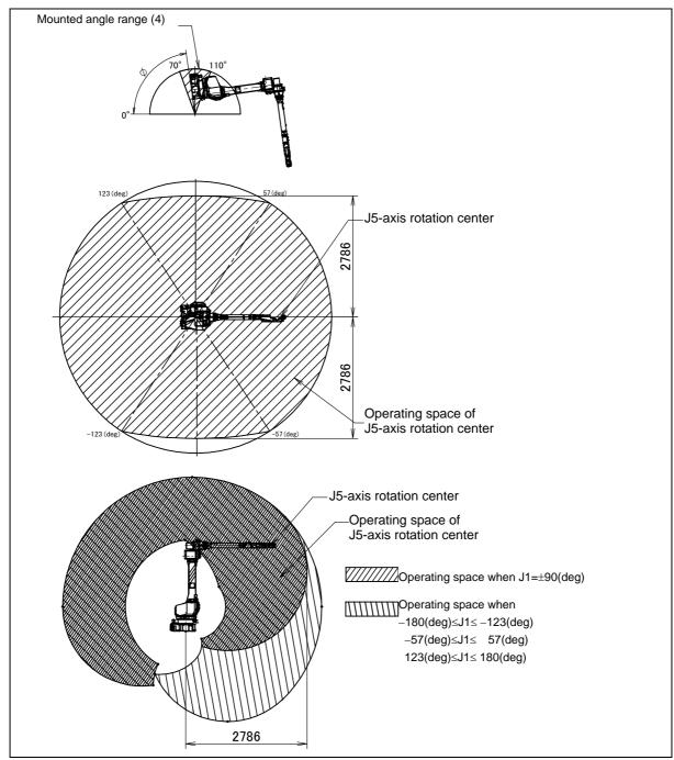
Fig. 3.7 (h) Operating space for mounted angle range (4)  $(70^{\circ} < \phi < 110^{\circ})$  (M-710*i*C/12L)
