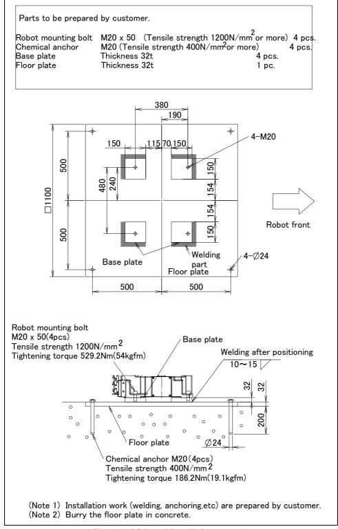
Fig. 1.2.1 (a) Actual installation example
