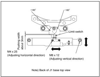
Fig. 6.4 Adjusting J1-axis limit switch (option)
