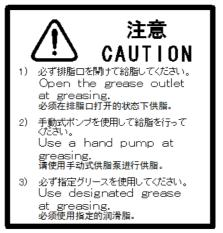
Fig. 10 (a) Greasing and Degreasing Label
