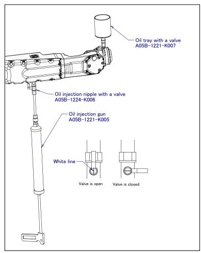
Fig. 8.3.2.3 (c) Oil injection by oil gun
