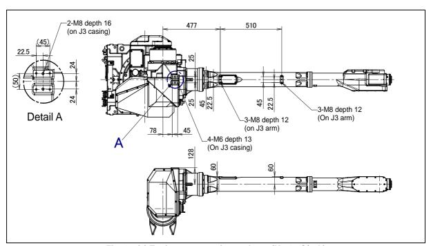
Fig. 4.2 (a) Equipment mounting surfaces (M-710iC/20L)
