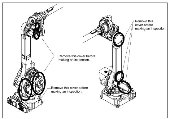
Fig. 8.2.5 (a) Inspection points of the mechanical unit cables
