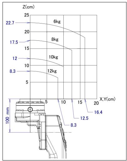
Fig. 3.4 (b) Wrist load diagram (M-710iC/12L)
