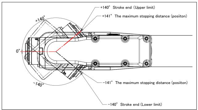
Fig. 3.3 (f) J5-axis motion limit (M-710*i*C/20L/20M)
