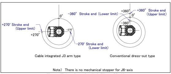
Fig. 3.3 (i) J6-axis motion limit (M-710iC/12L)
