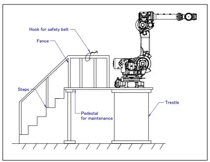
Fig. 3 (c) Pedestal for maintenance
