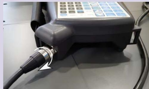
Rotate the teach pendant cable until it is seated. Then, spin the end of the connector until it is threaded on tight. Wiggling the connector might let you tighten it more.
